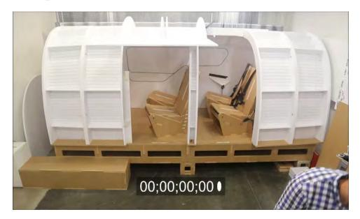
Hundreds of tests performed to optimize sizing, step-up, grab handles, and luggage loading. The end result was more like a car than an aircraft.
